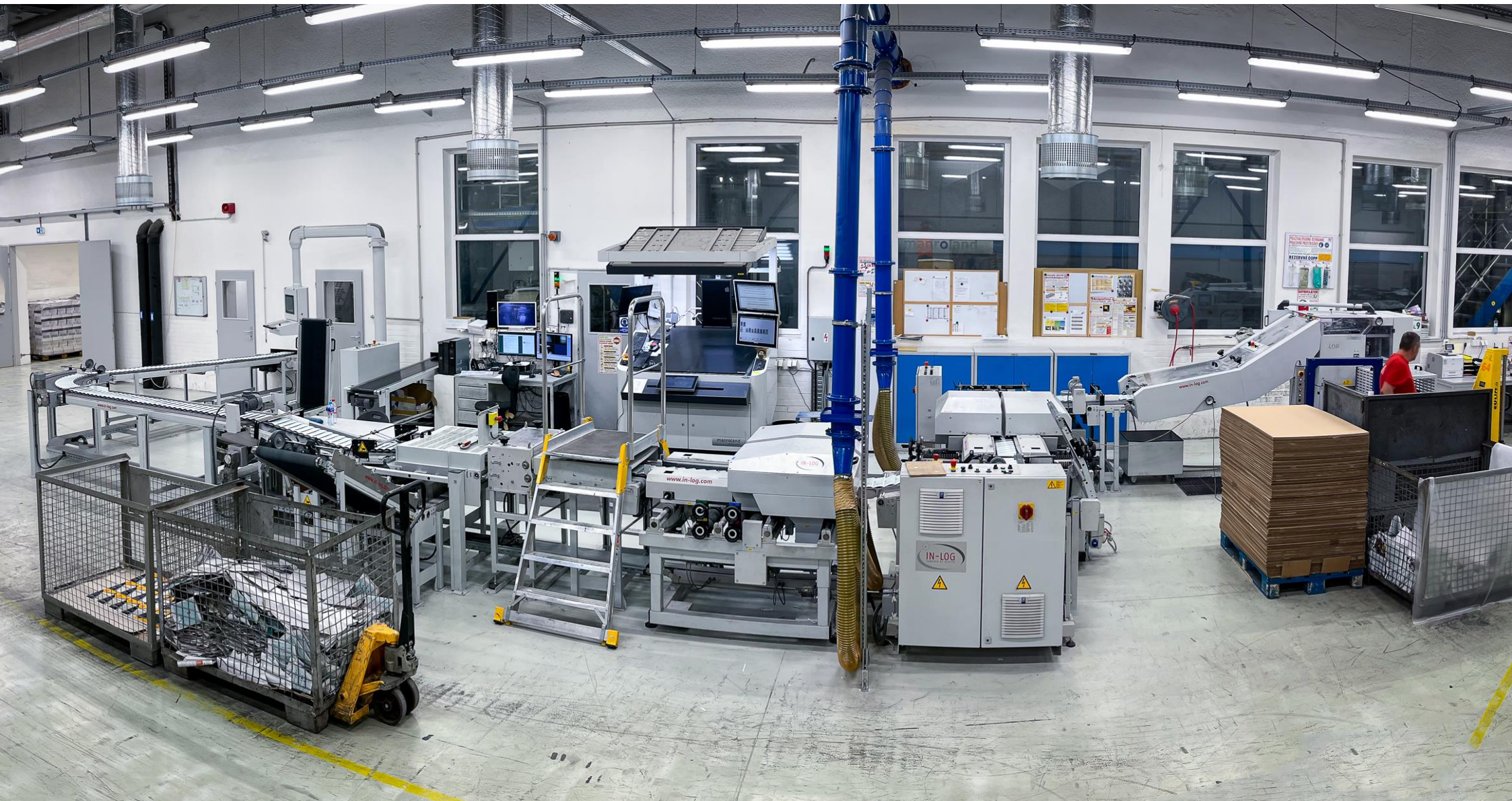
▲ View of the Post Press area – simple line layout with quick access for the press operator to the delivery conveyors as well as to all machines.
