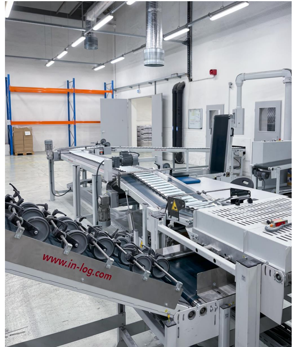
▲ Central waste ejection and stream aligner are placed after merging the magazine & tabloid delivery into one stream.
