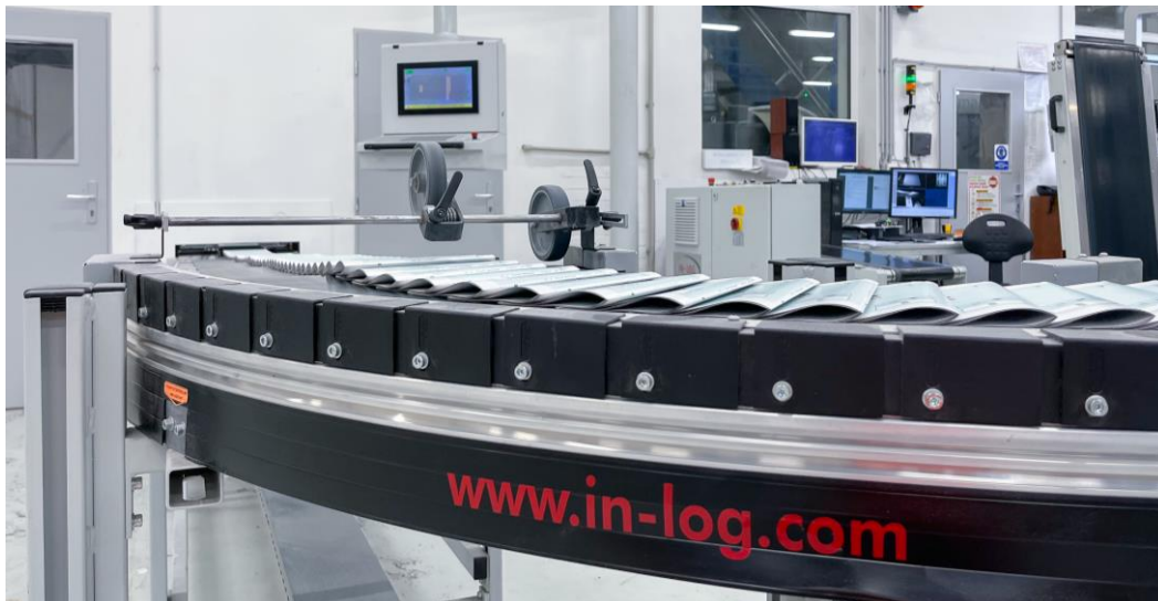
▲ After the flow turn the tabloid and magazine deliveries are merged.
