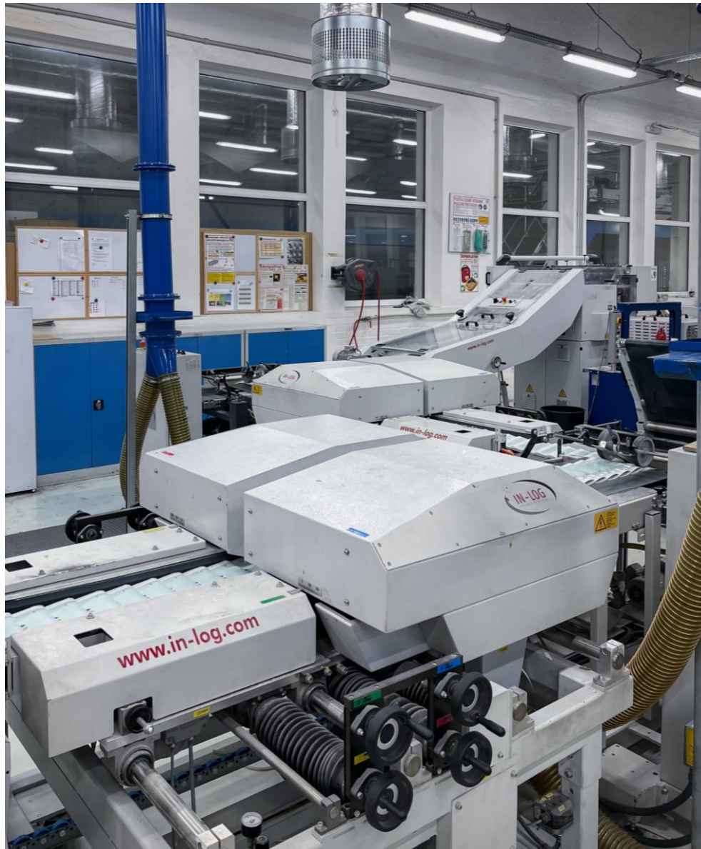
▲ Head / foot trimming is done in the first trimmer.
