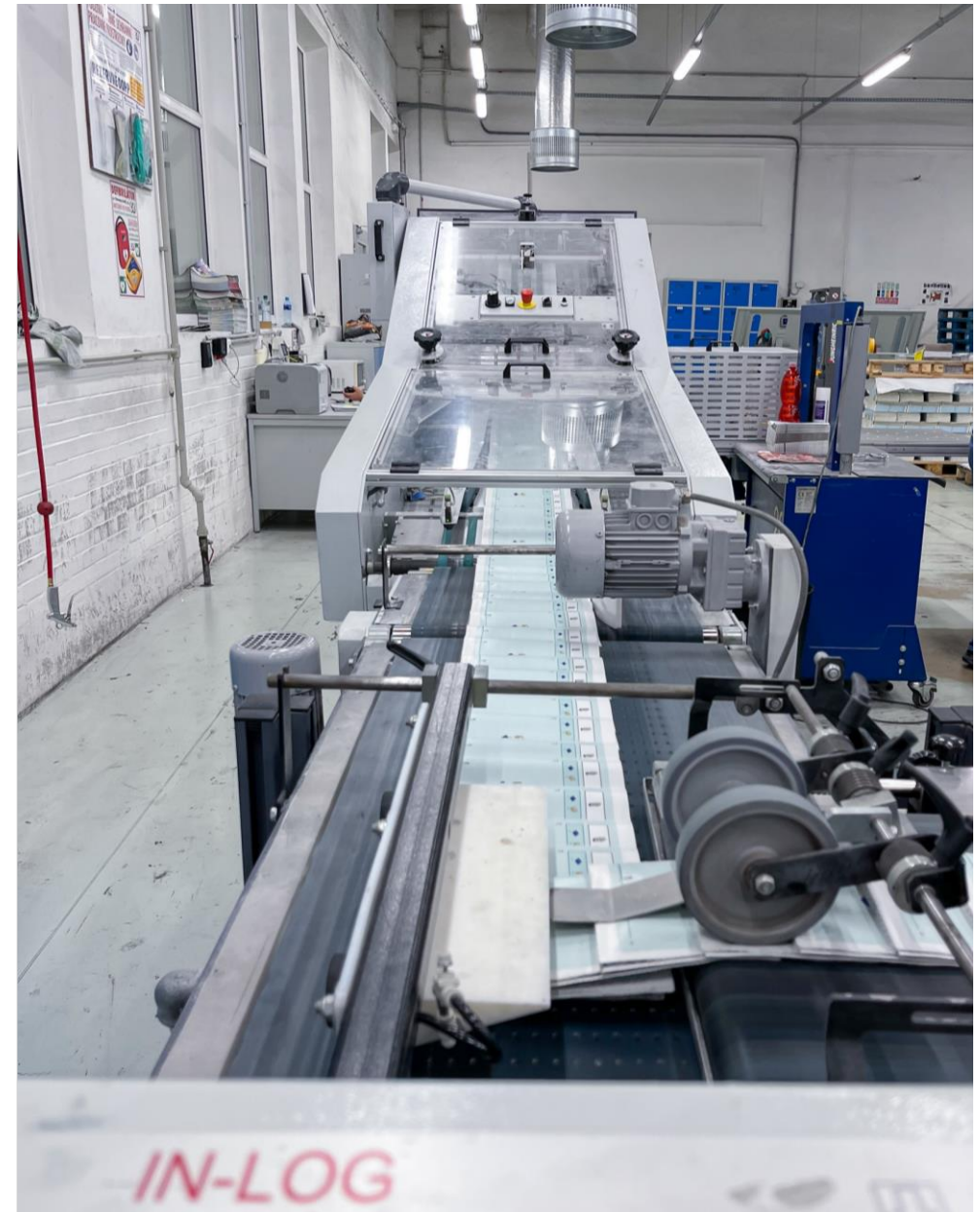
▲ All copies enter the compensating stacker "spine leading".
