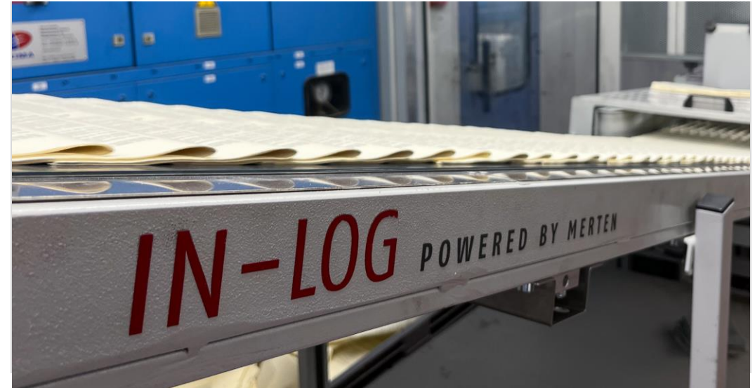
▲ The shingled stream descends to floor level for further processing
