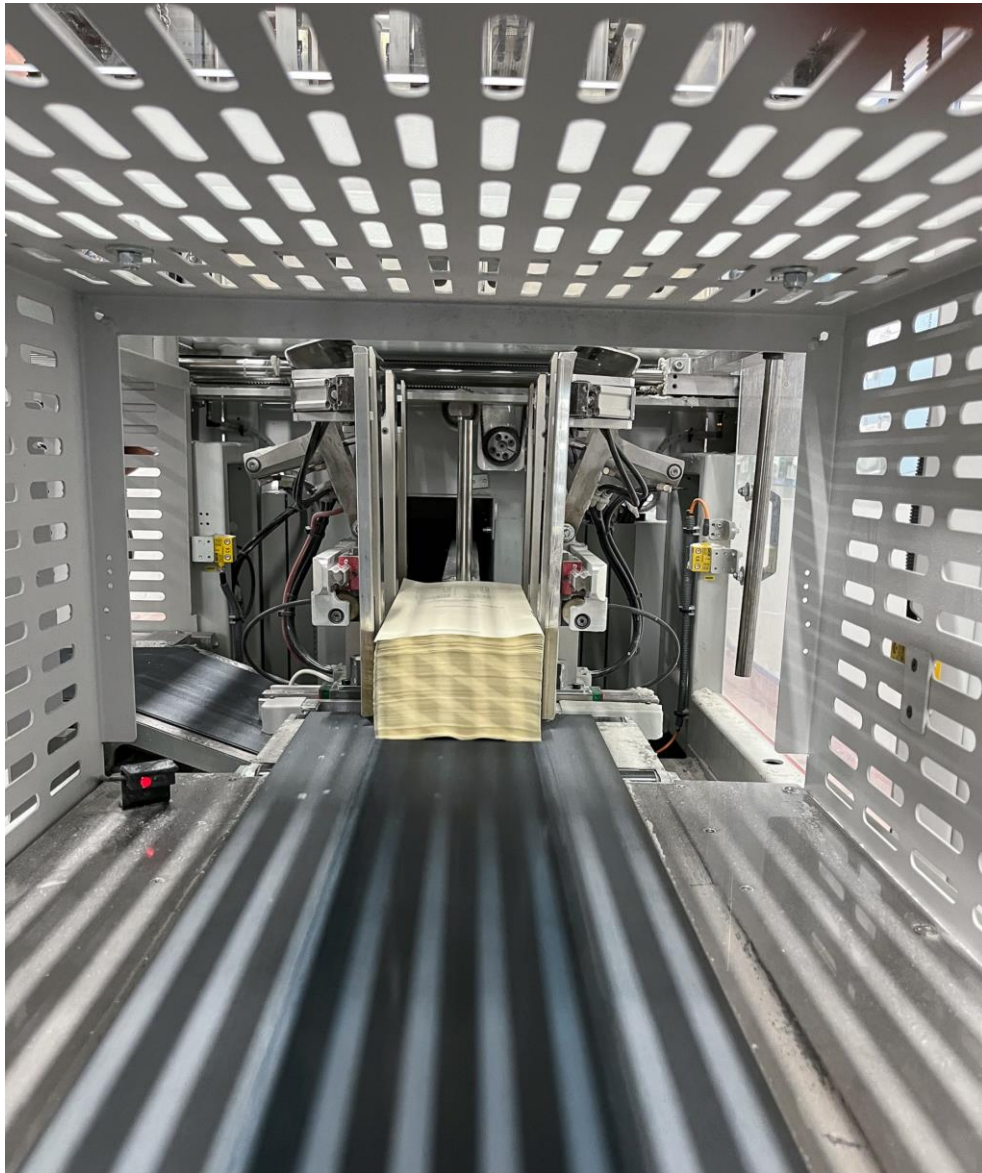
▲ The lift technology makes sure we have a no drop pre-stacking and a minimal dropping height between upper bin and turntable.
