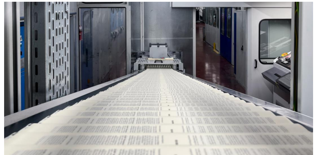
▲ The shingled stream leaves the sound protection wall for further processing in the trimmer and lift stacker
