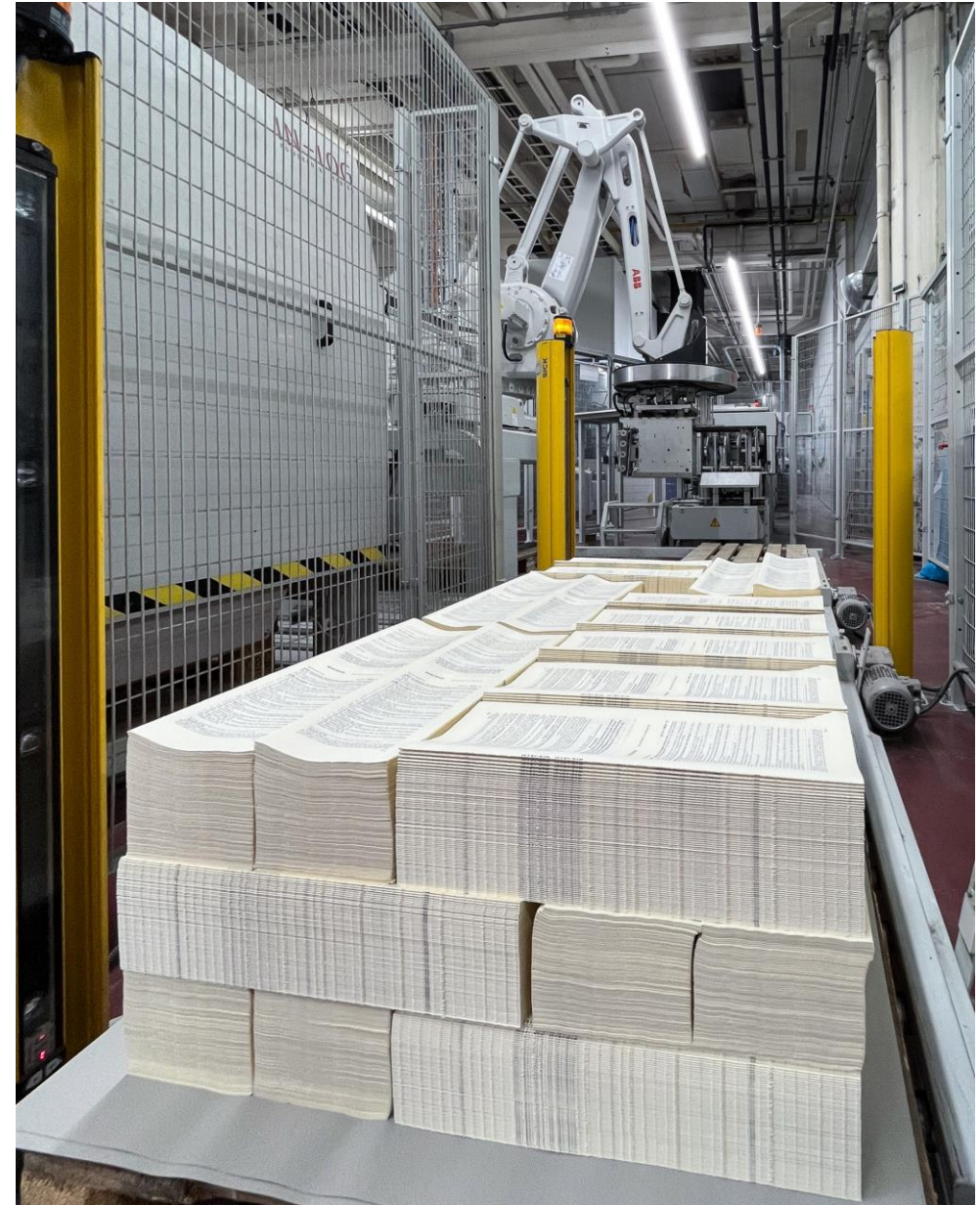
▲ Nicely built pallets with perfect bundles – best for the further processing on a perfect binder or a sewing machine.
