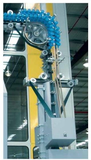
Infeed station and vertical conveying section
