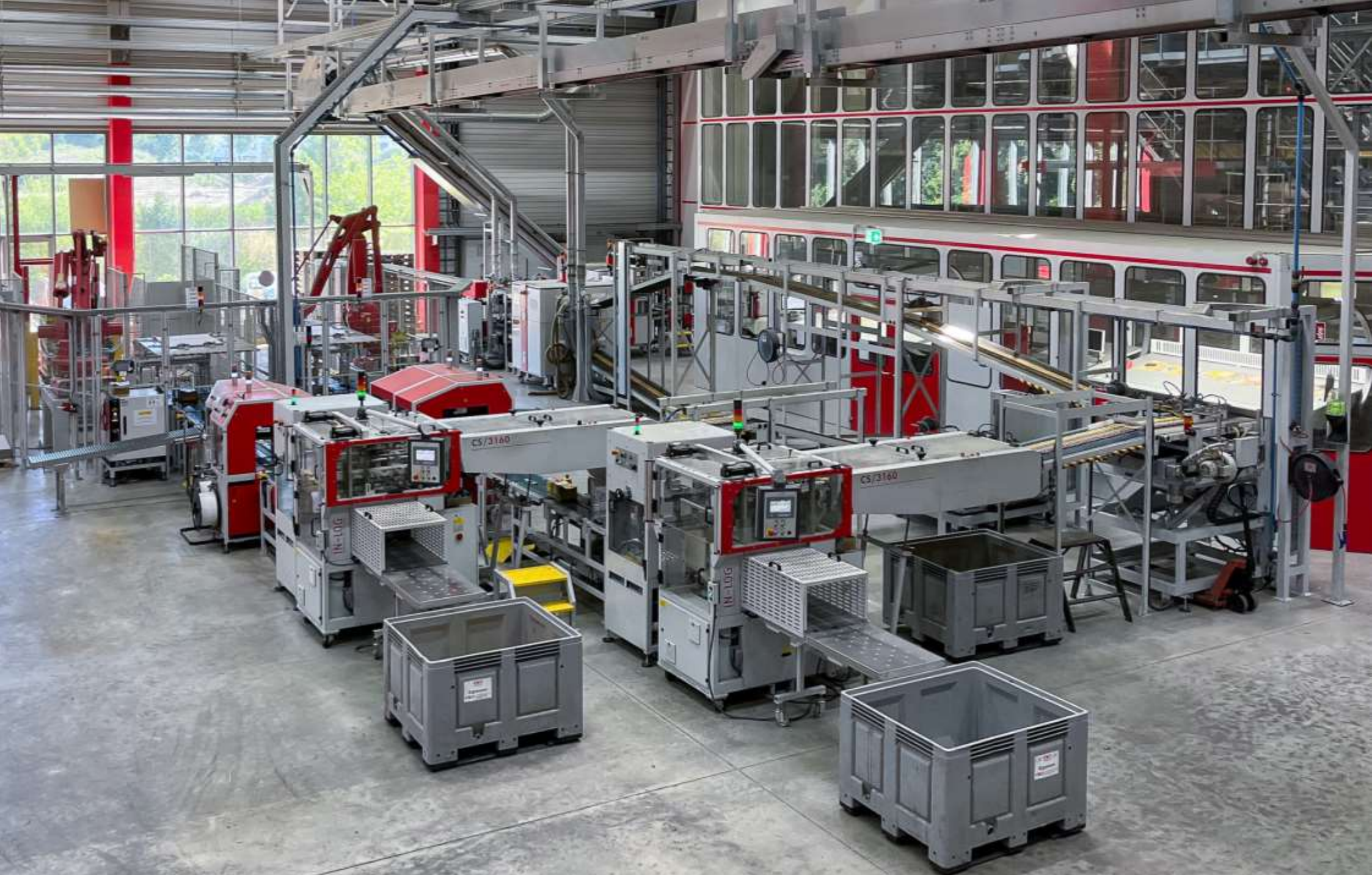
▲ The „Beast” – a 96p Lithoman web press with two folders, able to deliver more than 5 million of inserts per day. Behind the folders a fully automated Post Press System transforms the shingled streams in trimmed and stacked bundles, nicely palletized.
